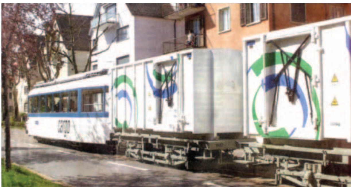
Cargo Train in Zurich – a train with two trailers converted into a mobile rubbish collection station – a pilot project has been collecting rubbish in the city's peripheries
