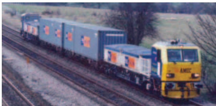
IRIS trials using an adapted Railtrack multi-purpose vehicle
